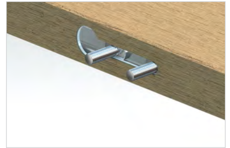
Setting up the second flange bolt.
