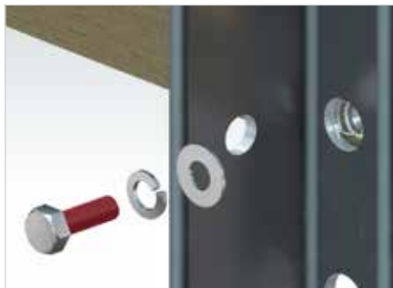
Installation of the supporting structure
