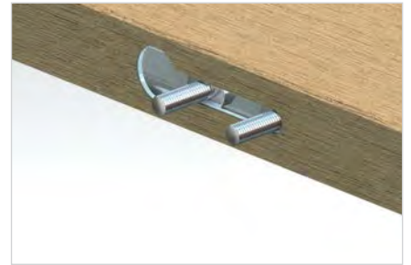
Setting up the second flange bolt.
