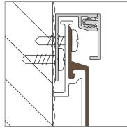
The Geolam 2-Piece starter (J-trim)\* can be used at the top to cover the screws if required
