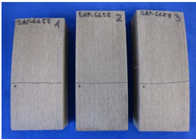
Image 2 – samples after 240h NSS
