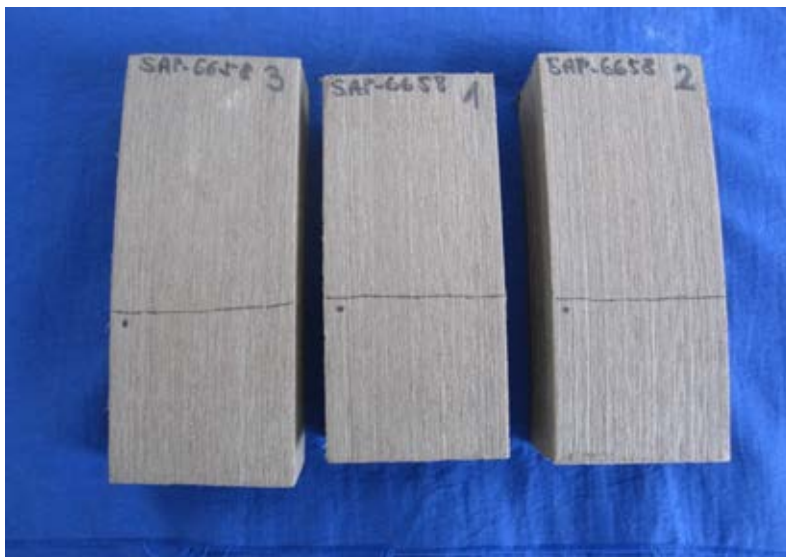
Image 5 – samples after 1000h NSS
